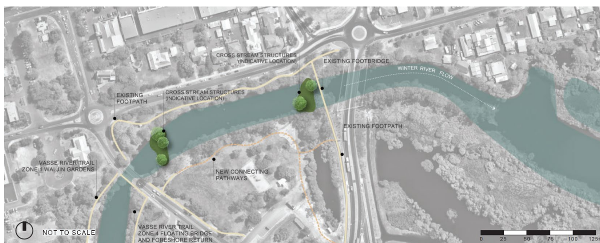
Figure 14. Plan view of the cross-stream structures showing isolated waterbody (between the two structures) during summer. Location is indicative only and would be finalised during detailed design phase.
