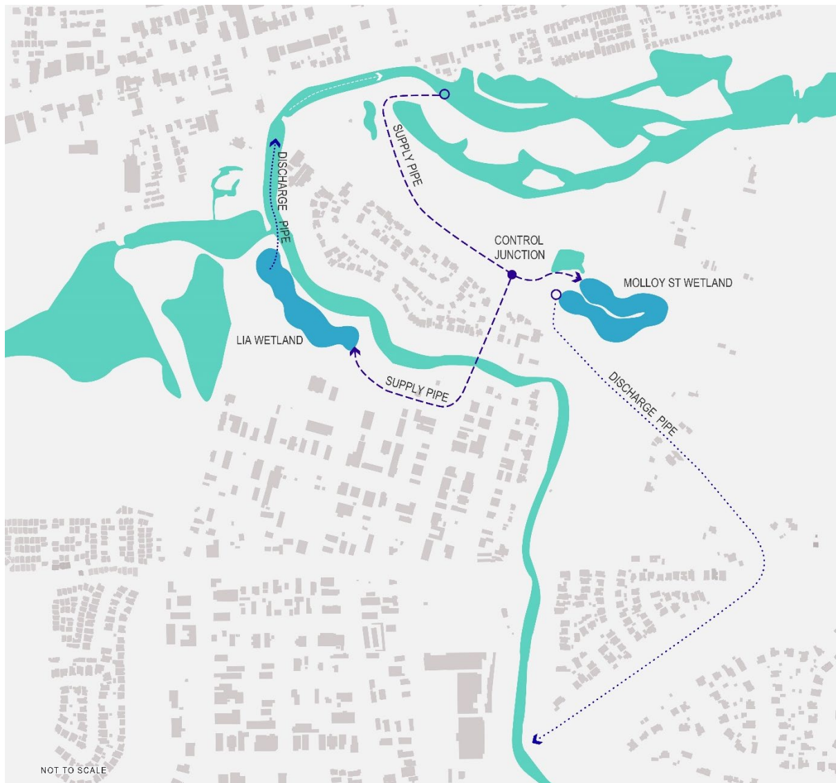
Figure 13. LIA and Molloy Street wetland combined pipework.
