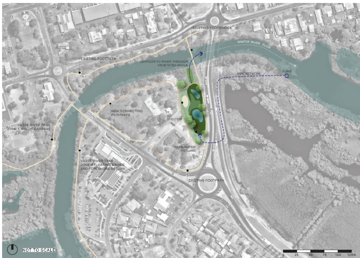
Figure 18. Rotary Park enhanced wetland concept. Showing treatment area, and treatment swale.
