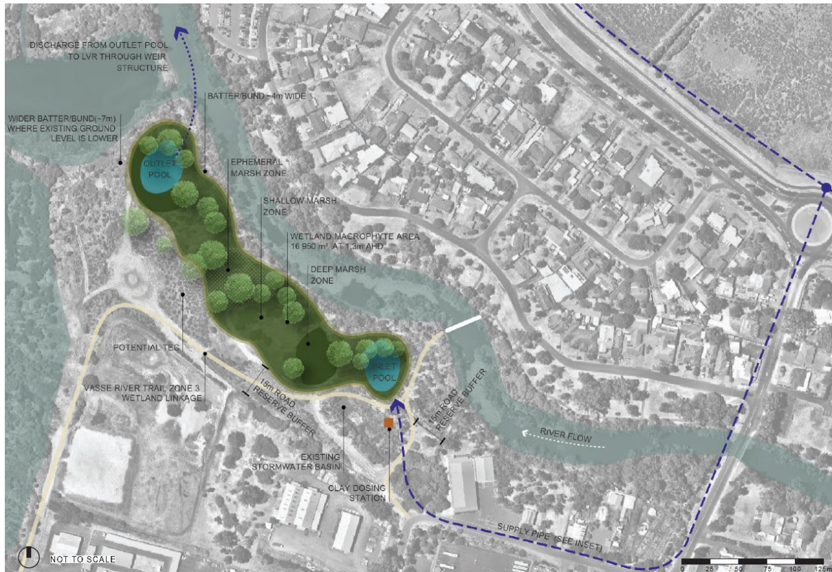
Figure 9. LIA constructed wetland concept. Showing treatment area, macrophyte zones, and proposed pipe network.
