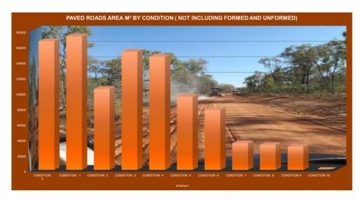
The above chart shows the condition breakdown for paved roads only (not including formed and unformed) which drives the annual re-sheeting program. Roads sitting in the condition eight and nine and ten ratings are those which are scheduled for re-sheeting. These will be rectified through the current re-sheeting program and do not indicate any current back log of works for unsealed roads.
