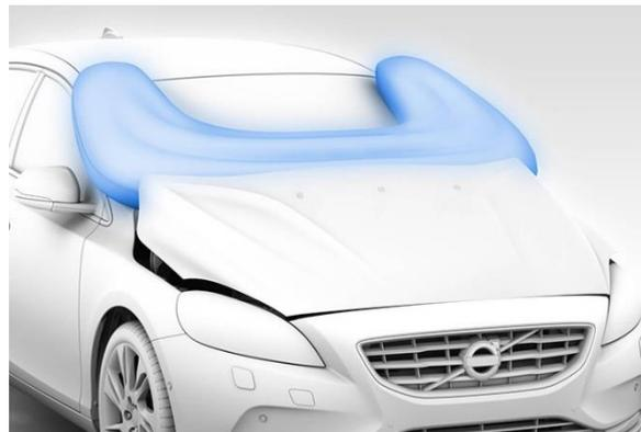
Rescue personnel must utilise existing safe working practices when working near other gas-driven inflation and propulsion systems, including identification and avoidance of component parts. For Pedestrian Protection Systems, these are located near the bonnet hinges and can be identified by similar markings and inserts to Supplementary Restraint Systems (SRS) located near the windscreen wipers.
