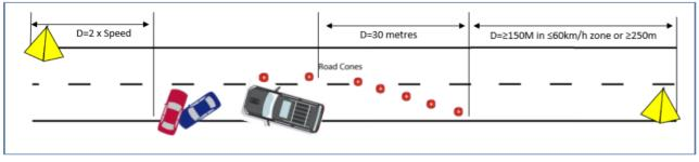
Figure 2 – Road Traffic Control Measures in support of Incident and Fend-Off Position (where practicable)
