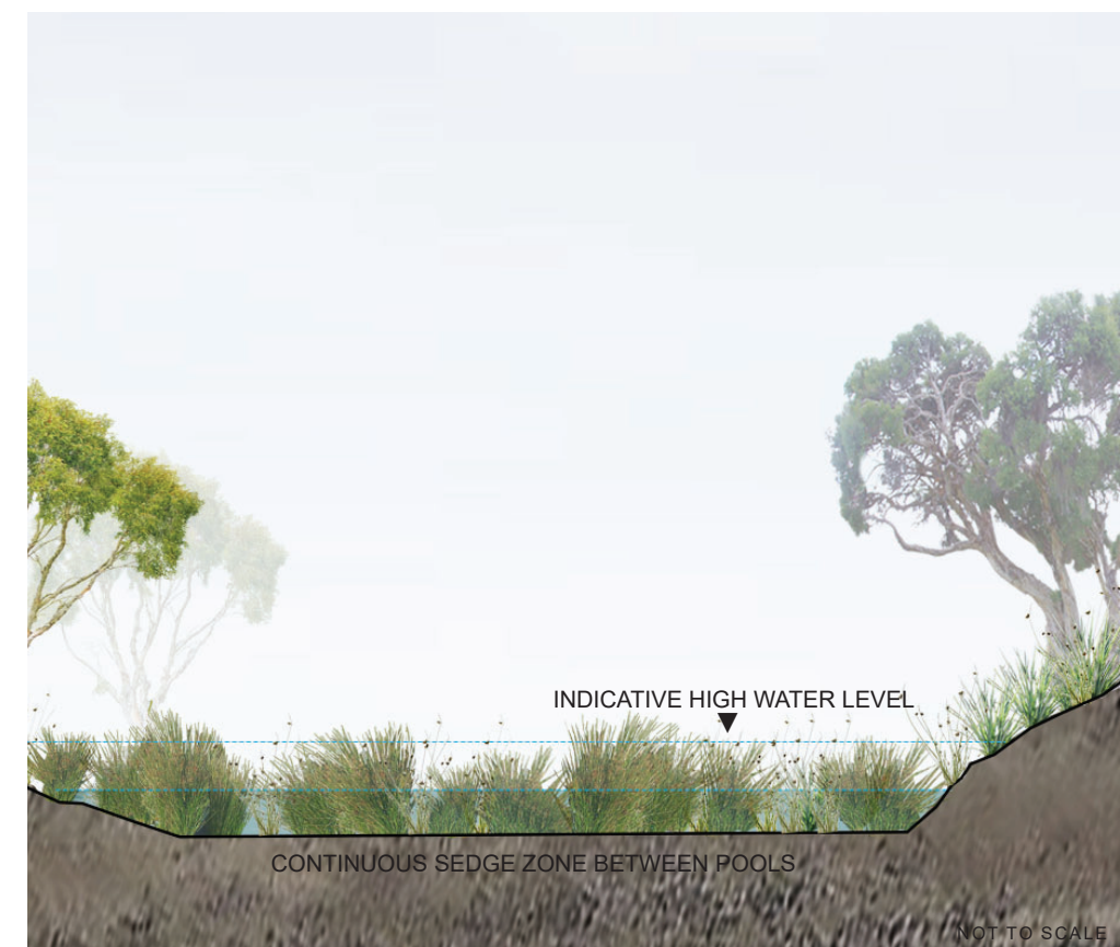
INDICATIVE CROSS SECTION THROUGH SEDGE ZONE
