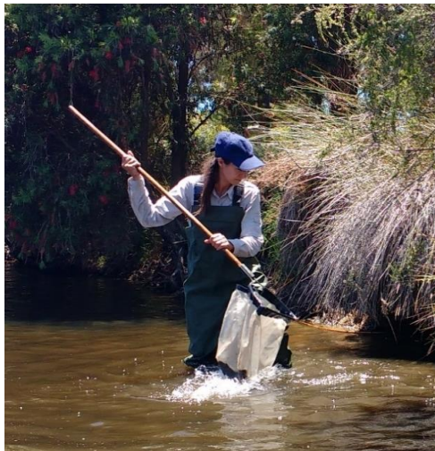
Figure 9: Sampling of invertebrate organisms with a fine sweep net.
