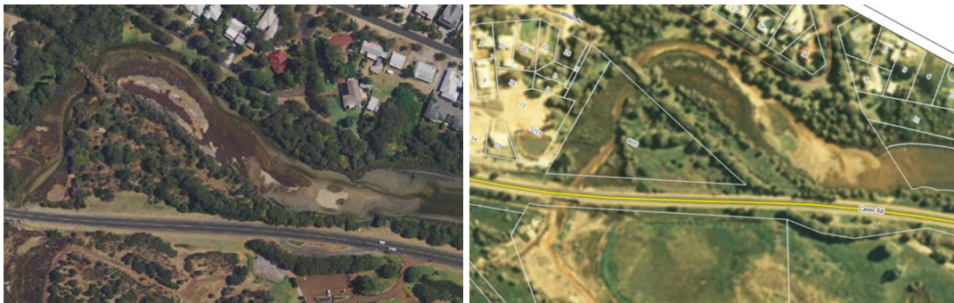
Figure 7. Comparative aerial photographs of sediment deposition in Toby Inlet downstream of Caves Road, from 2018 (left) and 1997 (right).
