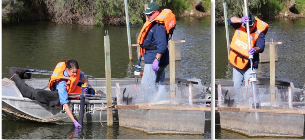
Figure 8: Sediment sampling with a hand coring device.
