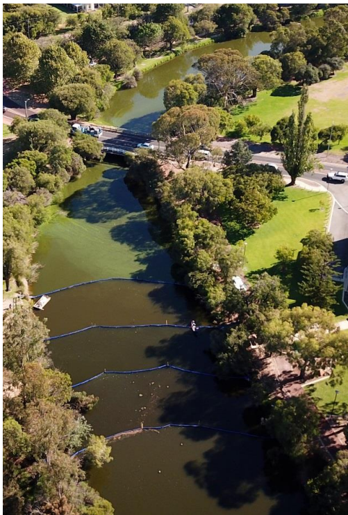
Figure 14: Aerial view before clay application in February 2018. Algal blooms in the Lower Vasse River typically start to develop at the downstream end between the weir boards and the causeway bridge before spreading further upstream.
