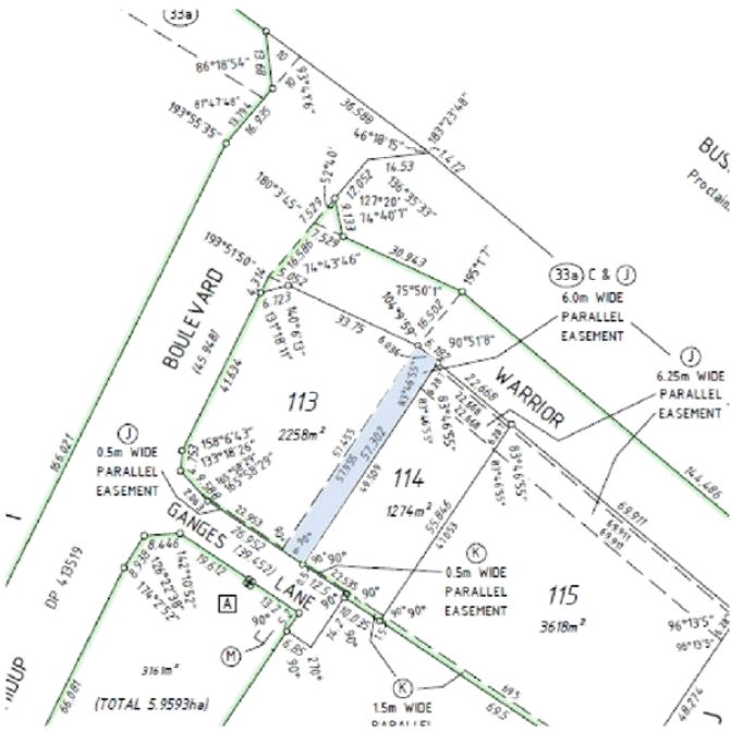
Figure 2 Lot 113 showing easement. The easement is against the wall of the building on Lot 114.
