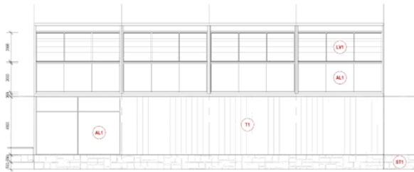
05 BUILDING 02 EASTERN ELEVATION NEW MIXED USE - SCALE 1:100
