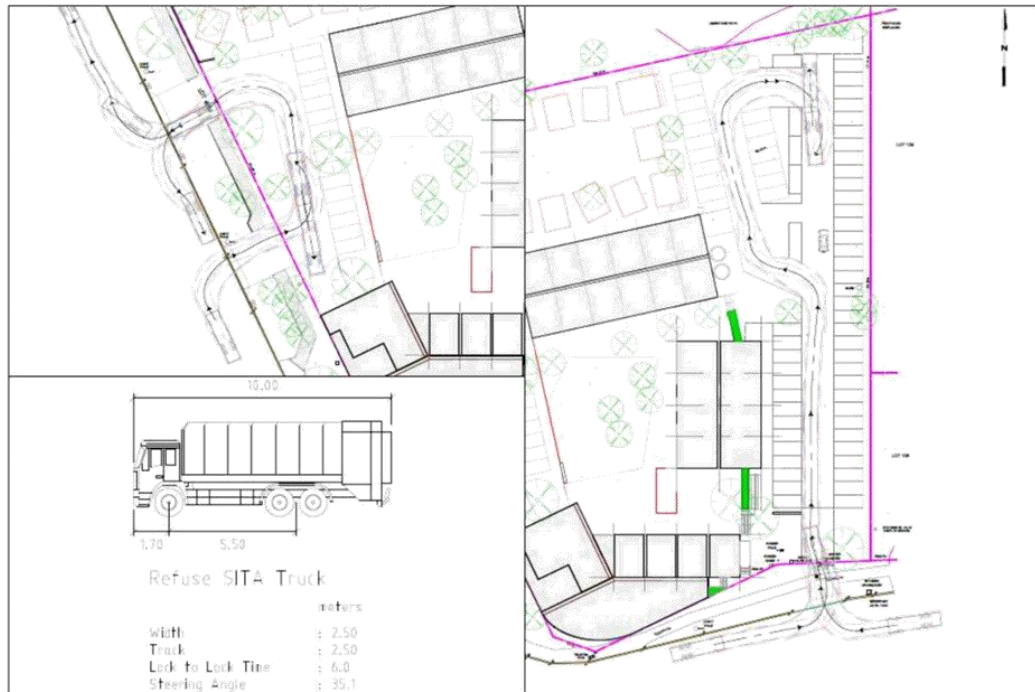
Figure 4: Swept path analysis showing access for waste collection vehicles to service bin stores 1 (RHS) and 2 (LHS)
