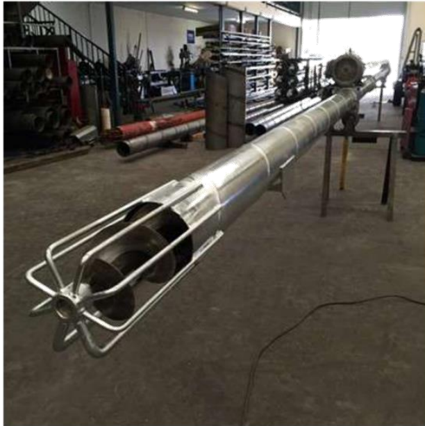
'Spent grain' silo auger
