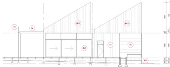
03 BUILDING 02 SOUTHERN ELEVATION NEW MIXED USE - SCALE 1:100
