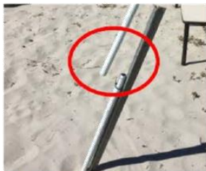
Only the bottom part of the leg is attached to the star picket anchor
