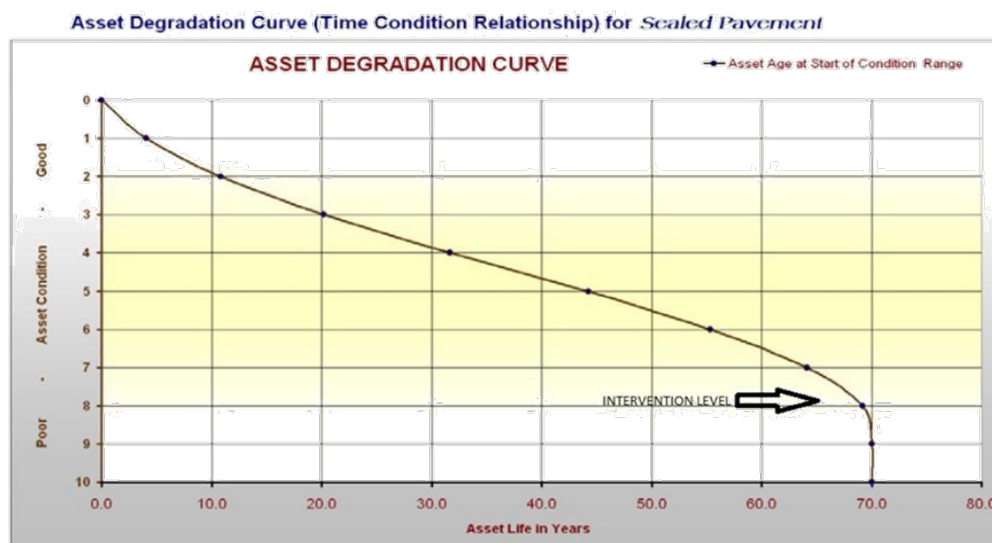
Chart 1. Typical Degradation Curve for Sealed Pavement.
