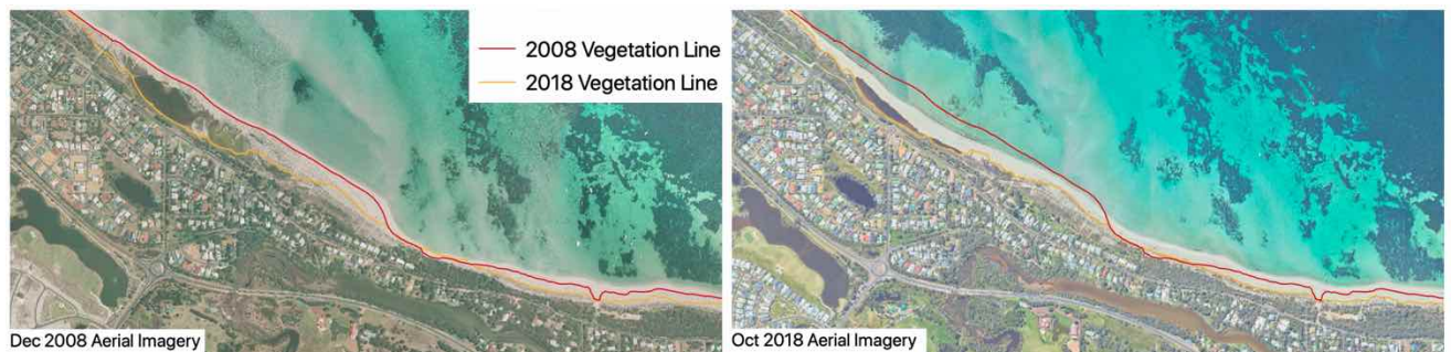
Figure 7.1 Dunn Bay Bar in 2008 (left) and 2018 (right) showing variability of sediment supply
