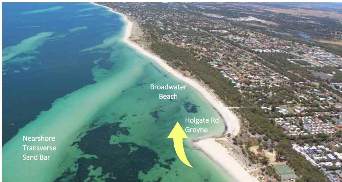
Figure 1.3 Broadwater Beach - Holgate Road Groyne. In 2020 this structure was refurbished and shortened by 20m to improve supply of sand to Broadwater Beach
