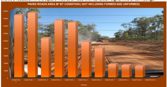
The above chart shows the condition breakdown for paved roads only (not including formed and unformed) which drives the annual re-sheeting program. Roads sitting in the condition eight and nine and ten ratings are those which are scheduled for re-sheeting. These will be rectified through the current re-sheeting program and do not indicate any current back log of works for unsealed roads.
