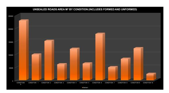
The chart above shows the current condition profile (zero very good, ten very poor) of the unsealed roads following the inspections. This chart includes 'unformed' (also known as unmade or unconstructed) roads which are essentially roads that provide some form of access but have not been improved or shaped (formed) in any significant way. Re-sheeting works are generally only scheduled for formed roads unless there is specific need to improve the service level of an unformed road.
